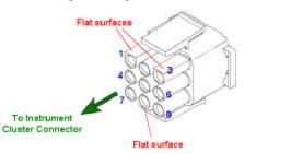
Pins numbers are also shown on the diagram in blue. These pins are not easily removeable without a special tool, so check and re-check each pin carefully prior to inserting them into the housing. When the pins is fully inserted into the housing, you will hear a click.
