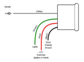
• BLACK -- connect to a solid chassis ground under the dashboard, or directly to the battery. You may need to expose the metal connection point under the dash by scraping or lightly sanding it. A ring terminal and a screw should work well in most cases.
