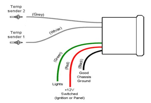
BLACK (Thick) -- connect to a solid chassis ground under the dash, or directly to the battery. You may need to expose the metal
