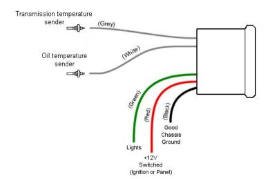
BLACK (Thick) -- connect to a solid chassis ground under the dash, or directly to the battery. You may need to expose the metal connection point under the dash by scraping or lightly sanding it. A ring terminal and a screw should work well in most cases.
