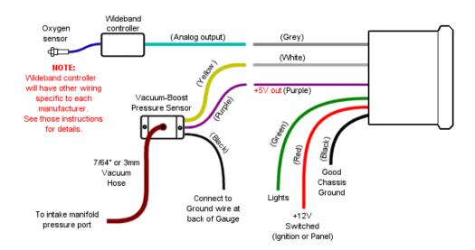
BLACK (on gauge) -- connect to the vacuum-boost pressure sender and then to a solid chassis ground under the dash or directly to the battery. You may need to expose the metal connection point under the dash by scraping or lightly sanding it. A ring terminal and a screw should work well in most cases.
