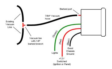
BLACK -- connect to a solid chassis ground under the dashboard, or directly to the battery. You may need to expose the metal
