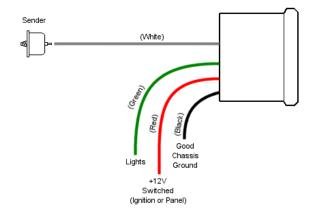
• BLACK -- connect to a solid chassis ground under the dashboard, or directly to the battery. You may need to expose the metal connection point under the dash by scraping or lightly sanding it. A ring terminal and a screw should work well in most cases.
